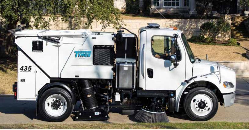
The Model 435 delivers street sweeping performance in a mid-sized package. With the Conventional Truck Package, the Model 435 has a payload of over 8000 lbs. and a overall sweeping path of 130 inches.
