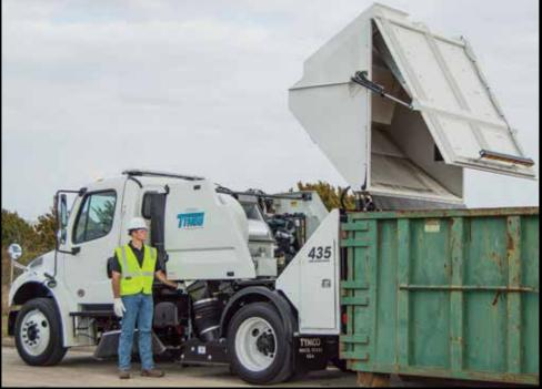
With the Conventional Truck Package, the Model 435 has a 82.5 inch dump height. (Most 30 yard containers are approximately 69 inches)
